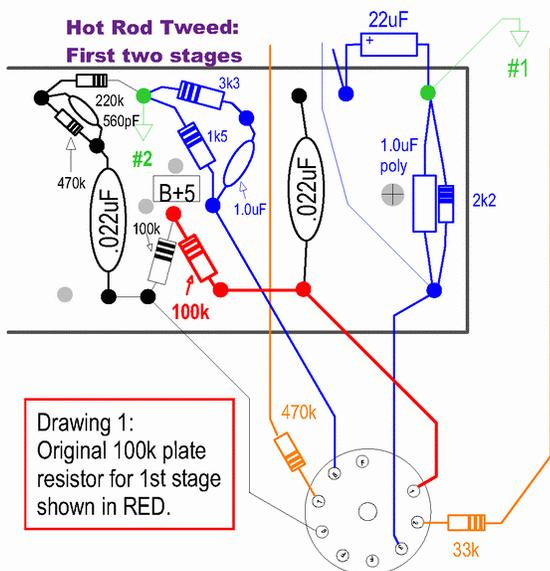
preamp. For prototypes, you could replace a 100k plate resistor with a 100k linear pot, with the wiper connected to the coupling cap (or tone stack) and the outer terminals connected to the plate and to the B+. (Most pots are not designed to be subjected to raw DC like this, so this is only a temporary measure to determine which pair of fixed resistors to use on each stage.)
