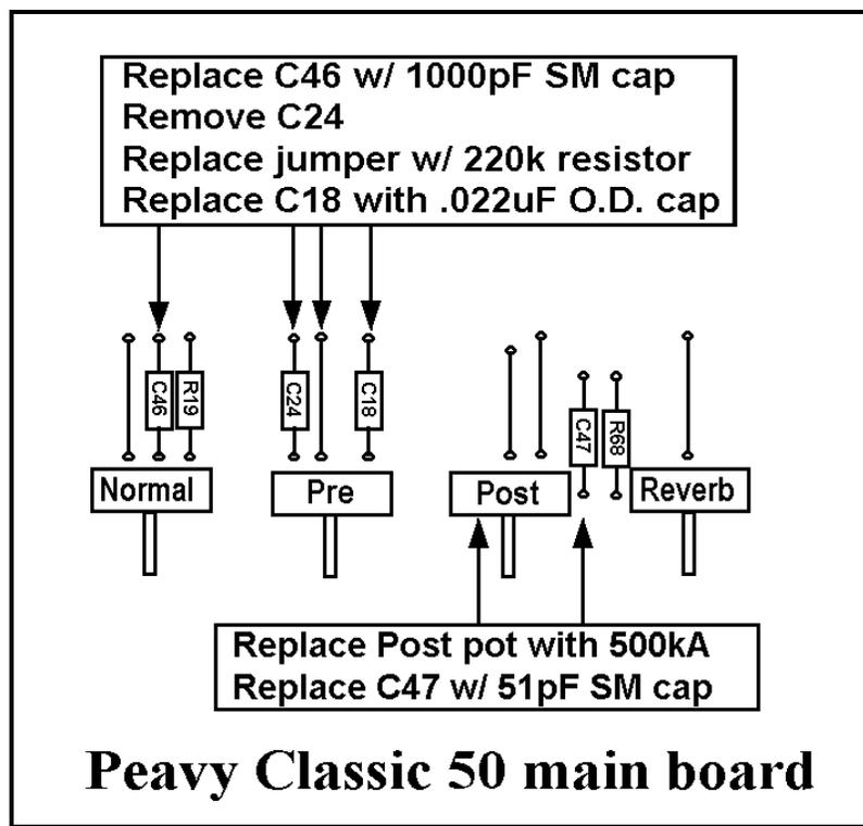
**Figure 3. Main board: channel volume controls**
