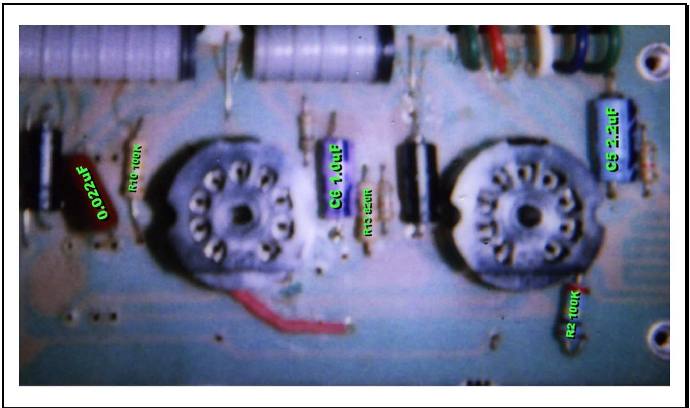
Figure 6. Component side of preamp tube board after mods completed.
