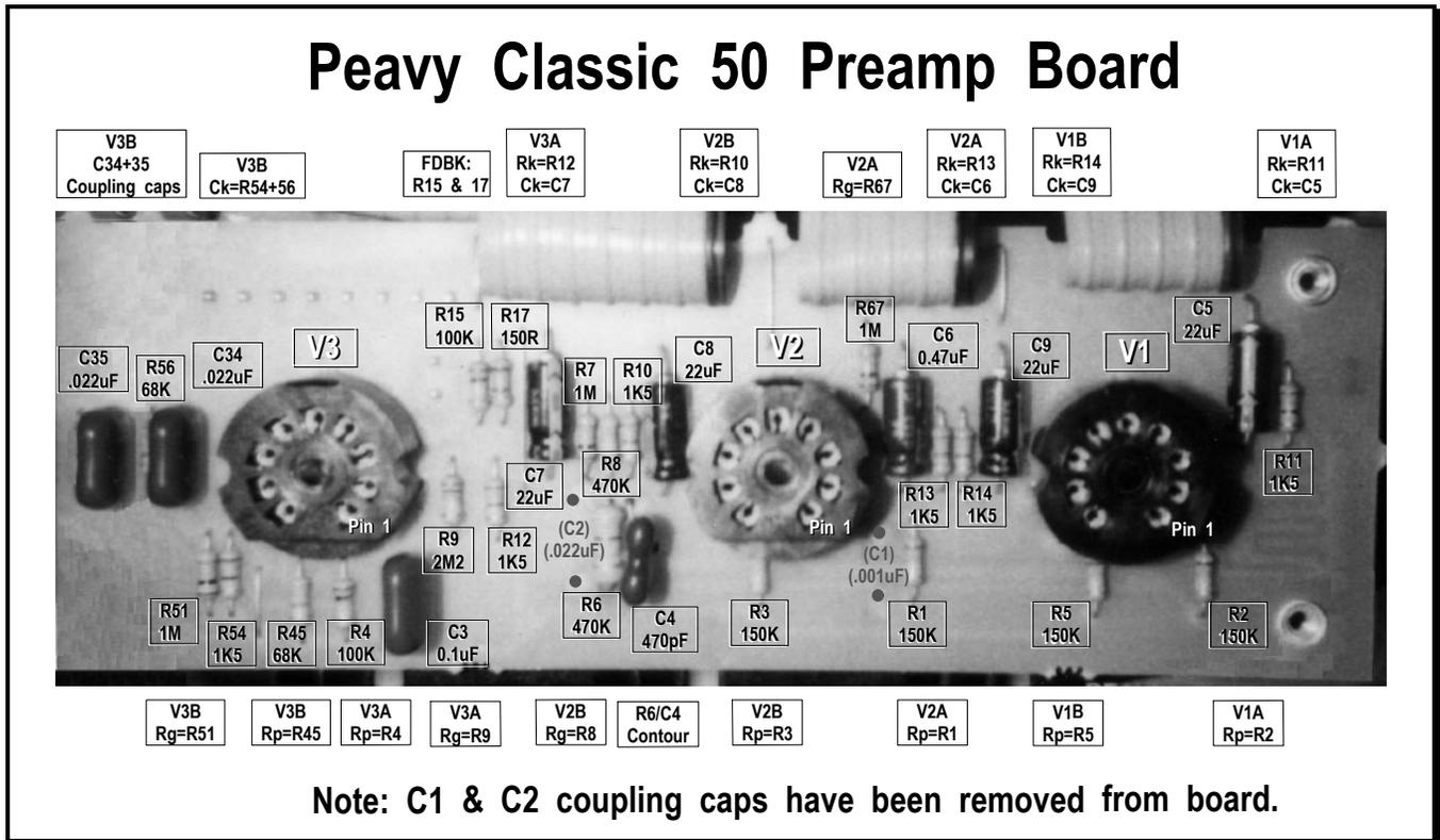
Figure 5. Component side of preamp tube board before mods begun.
