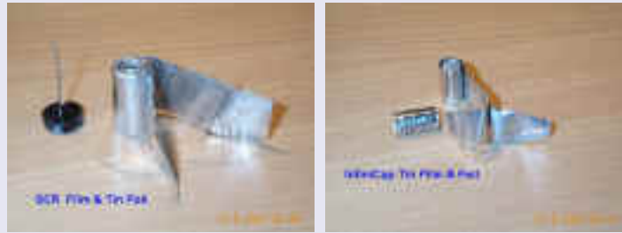
2 Tin Foil with 2 polypropilene Foil
